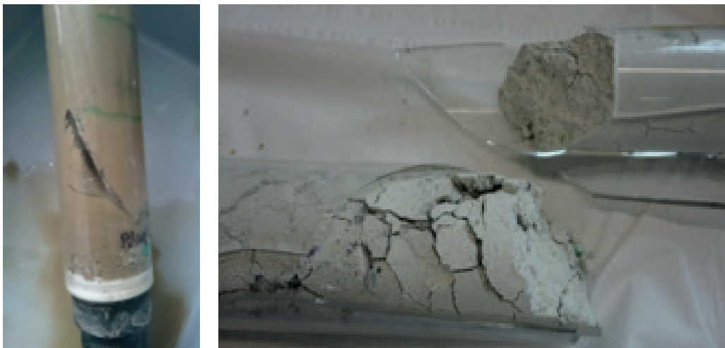
Fig. 1: left: heavily compacted, non-percolating mineral coal fly ash in the glass column of the percolation column procedure (DIN 19528); right: stabilised, non-percolating ladle slag in a shattered glass column
