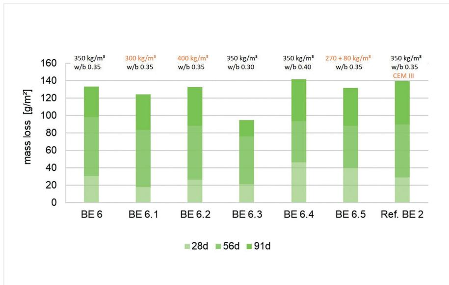
Figure 9: Mass loss of concretes BE 6 after 91 days of storage in  $H_2SO_4$
