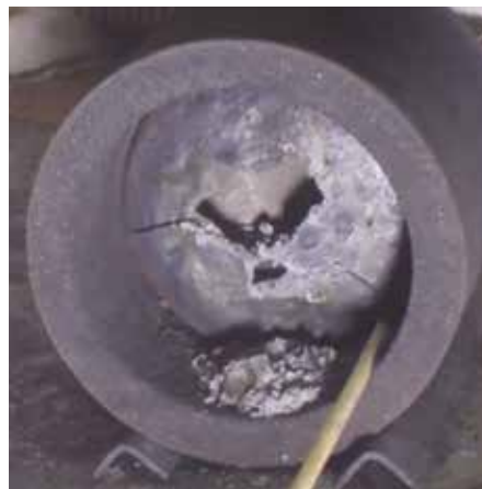
Figure 4: LF slag in a muffle furnace with a thermocouple disintegrating during cooling
