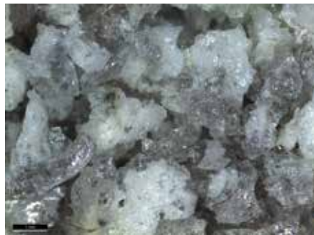
Acti 12 with 19.7 wt.-% Al_2O_3 , C/S = 1.70
