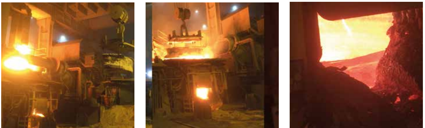
Figure 8: Charging the sandwich to the EAF
