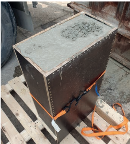
Figure 11: Production of the wall element in the ready-mix concrete plant of Spenner Herkules GmbH and its storage at FEHS-Institute
