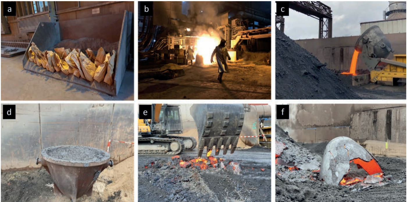
Figure 1: Operational tests for slag conditioning; a: bags with fluorspar, b: tapping of the molten slag, c: pouring the slag into the bed, d: empty slag pot, e: sampling of the bed sample, f: sampling of the rapidly solidified pot rim
