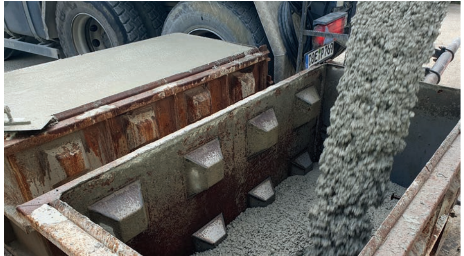
Figure 10: Production of "Lego bricks" in the ready-mix concrete plant of Spenner Herkules GmbH
