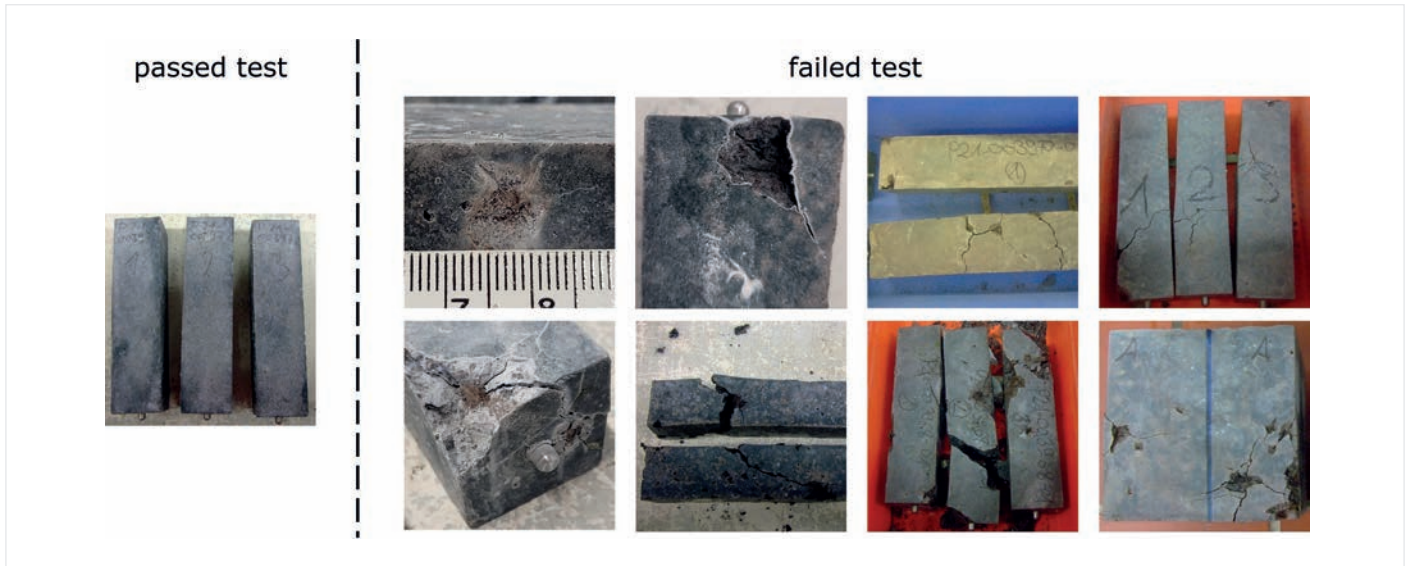
Figure 1: Visual assessment of volume stability. category 1 (left) = no damages = passed test. categories 2 to 5 (right) = damages of various intensities = failed test
